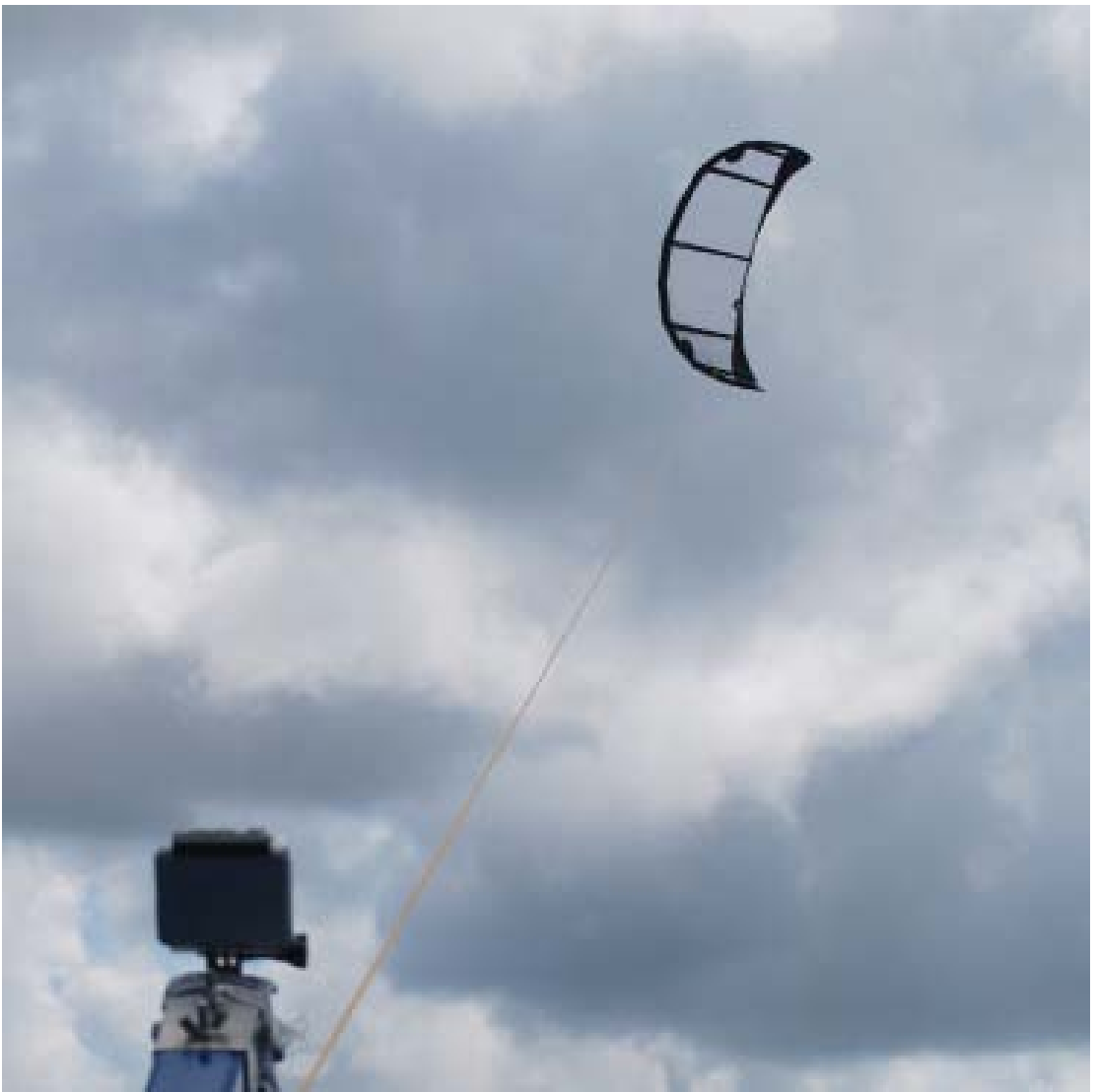
Fig 8: A 25 m 2 tube kite flying cross wind maneuvers observed from the ground station.
