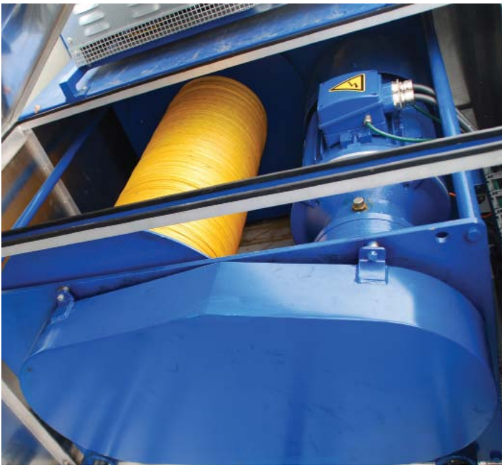
Fig 7: Cable drum and 20 kW electrical generator.
