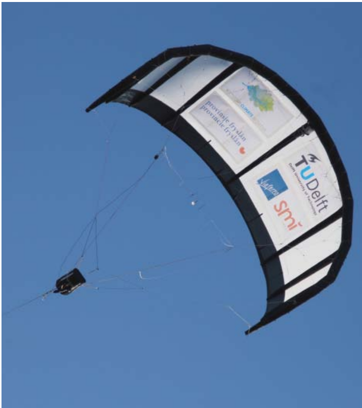
Fig 3: 25 m 2 Leading Edge Inflatable tube kite with suspended, tele-operated control unit.
