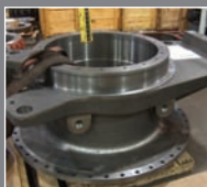
Planetary Gearbox Housing 7500 lbs
