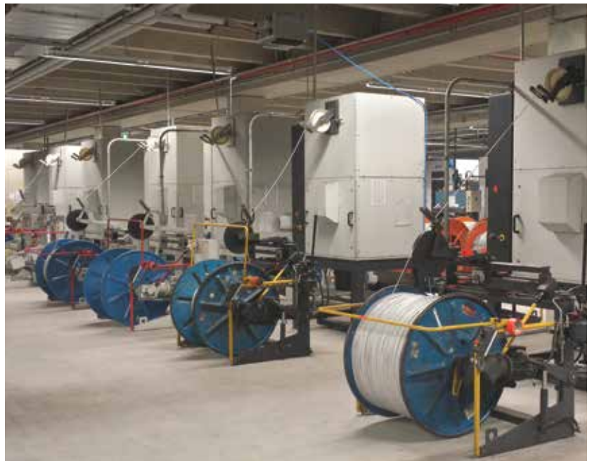
Helukabel manufactures its cables in both Germany and China. These cable machines are inside the Windsbach, Germany, factory. (Photos courtesy: Helukabel)
