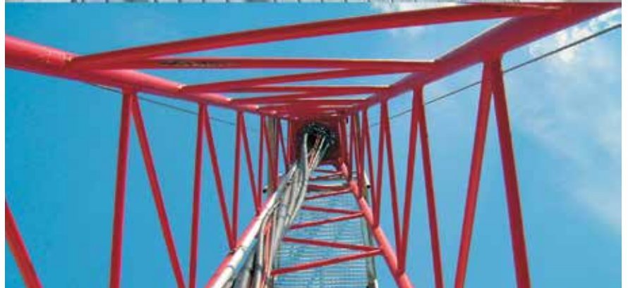
Helukabel can test up to 20 torsion cables at once in its 26-foot test tower that replicates actual nacelle rotational conditions 1:1. Cables are stressed up to 18,000 cycles and twist to the maximum of \pm 150 degrees per three feet
