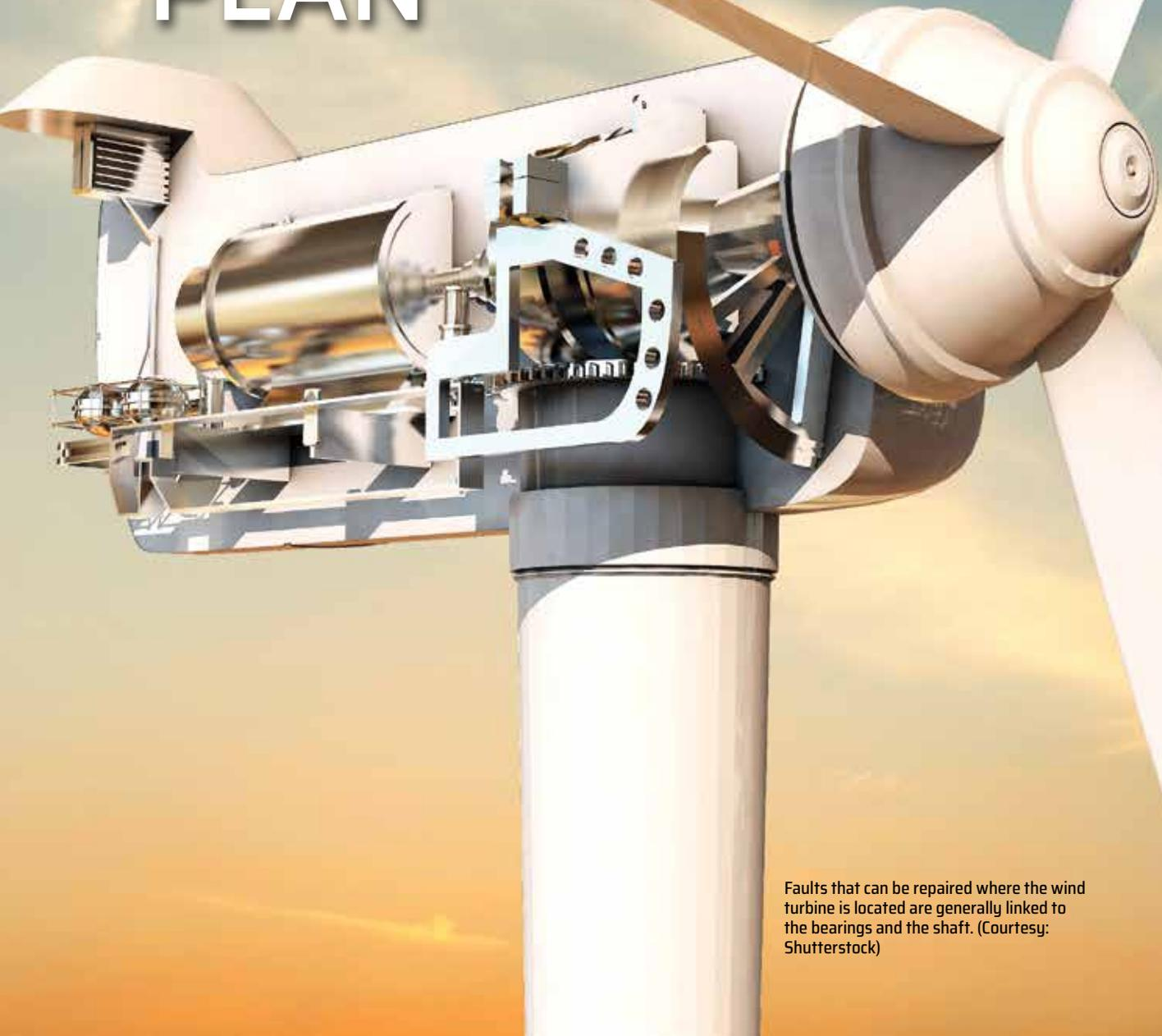
Faults that can be repaired where the wind turbine is located are generally linked to the bearings and the shaft. (Courtesy: Shutterstock)
