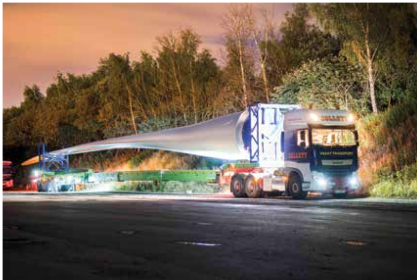
Super Wing Carriers can vary the trailer height, allowing Collett to raise the height of both the front and the rear of the trailer, resulting in each of the blades oversailing embankments and stone parapets when crossing bridges. (Courtesy: Collett)
