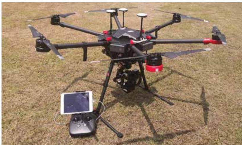
For a fully autonomous drone inspection in the market today, it means a drone should take off on its own, locate the turbine blades, complete the inspections, and land back at the starting point. (Courtesy: Clobotics)
