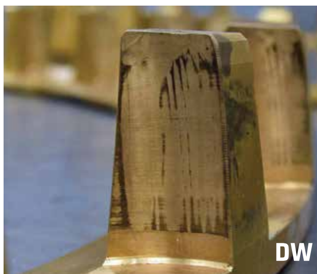
Figure 4: Brass cages offer extra strength in the toughest applications; no cage damage, and only minor discoloration, was observed in the 230/600-series Timken bearing. (Courtesy: Timken)
