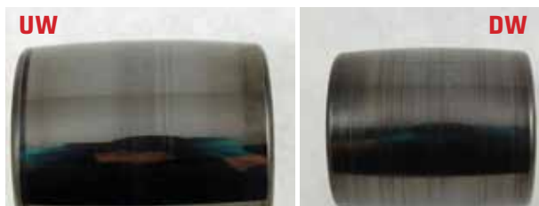
Figure 3: Both roller complements were in “very good” condition after operation and maintained their original profile. (Courtesy: Timken)
