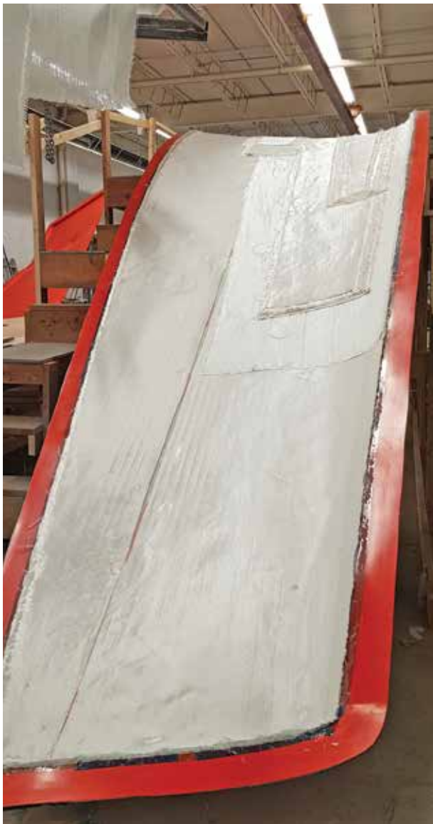
Manufacturing the PowerCone at CCI, showing structural layering of the fiber sheets. (Courtesy: Biome Renewables)
