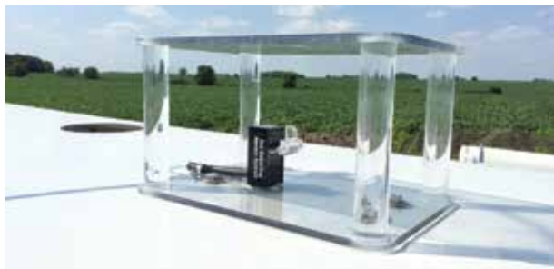
Figure 3: A shatterproof polycarbonate cage allows unimpeded airflow around a sensor body, protecting against falling chunks of ice and debris. (Courtesy: Vestas)
