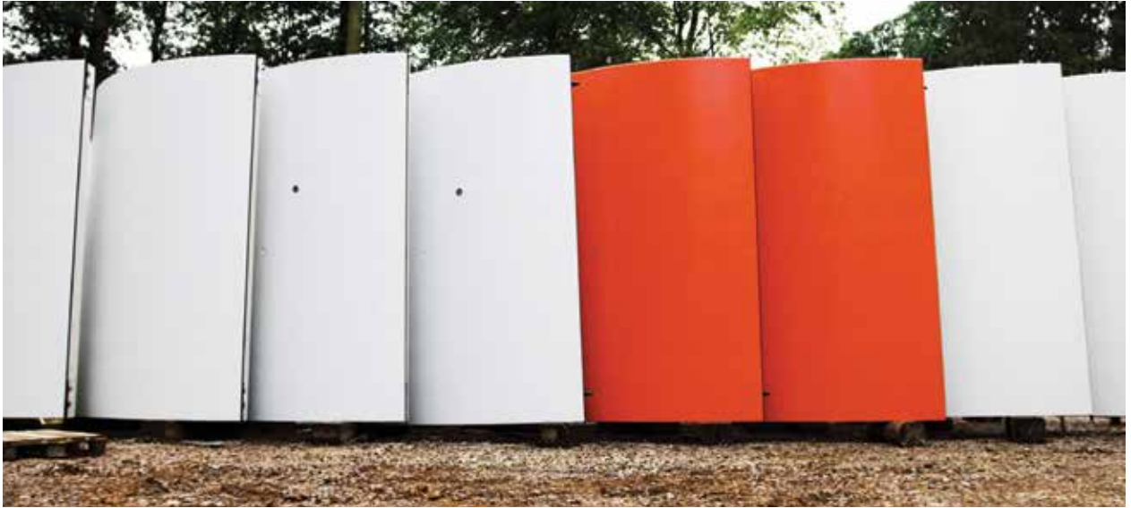
The concrete tower is prefabricated in segments that can be transported to a wind-farm site by standard trucks. (Courtesy: Max Bögl Wind AG)
