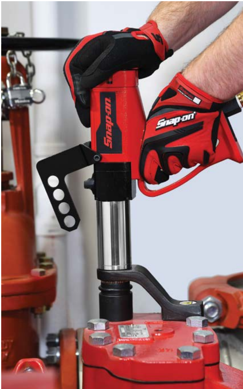
Torque multipliers are useful on wind farms or other remote jobsites, as they don't require electrical or pneumatic power sources. (Courtesy: Snap-on)
