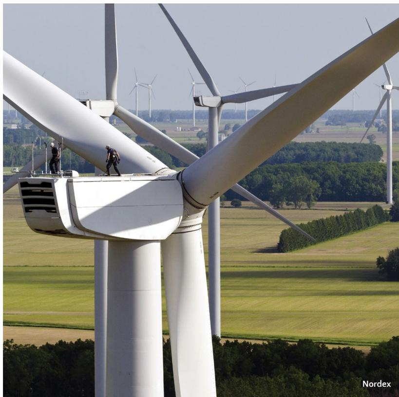
N117/2400 Gamma (2.4 MW) wind turbine
