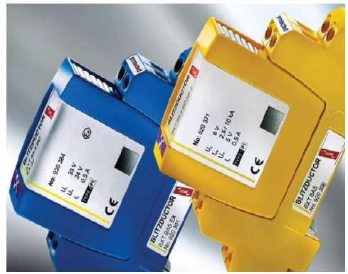
Fig. 3: Example of coordinated SPD for control circuits using coordinated gas discharge tubes and silicon avalanche diodes.
