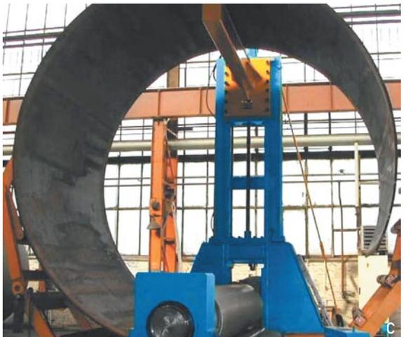
Figs. 3A-C: Three stages in the plate-bending process.
