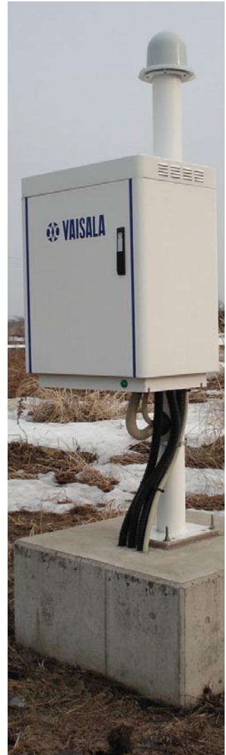
Fig. 3: Vaisala lightning sensor located in Tohoku, Japan, showing mounting pad, mast, electronics enclosure, and antenna assembly.
