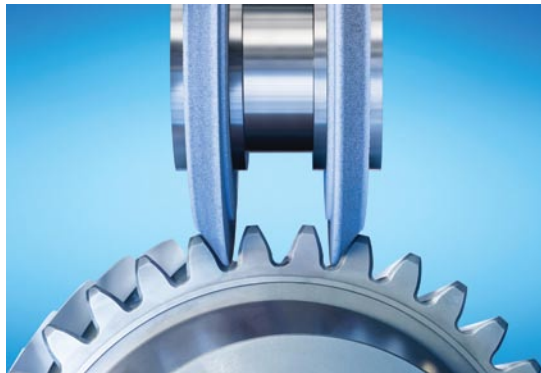
Fig. 2: Ideal for pinion gear production: Another OPTI GRIND variation shown here uses just the two outer wheels with each grinding a flank on separate gear teeth simultaneously. This variation reduces the radial infeed required, as compared to grinding conventionally with a single wheel.
