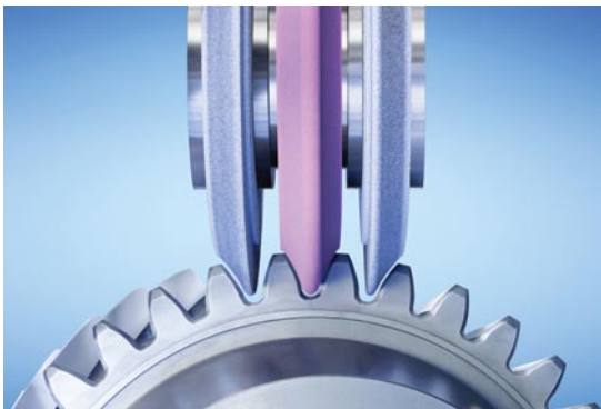
Fig. 3: Maximum OPTI GRIND surface finish quality: A third variation uses two outer wheels with an aggressive grit size to each rough grind a flank on separate gear teeth; then the middle wheel, shown here, with extremely fine grit size, finishes left and right flanks.
