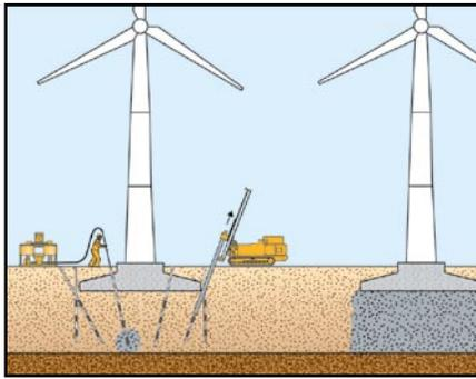
The volume of chemical grout needed to solidify a zone of granular soil is calculated by predicting the shape of the grout flow from the injection point determined by the subsurface conditions. In uniform granular soils, the grout typically flows radially from each port to create a spherical grouted shape. Based on a spherical flow model and the soil void ratio, the required maximum design volume can be calculated.
