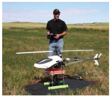
Fig. 1: The AutoCopter™ industrial strength, unmanned radio controlled helicopter (UAV).
