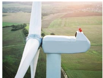
Fig. 3: The blades don't have to be repositioned for inspection using the AutoCopter.
