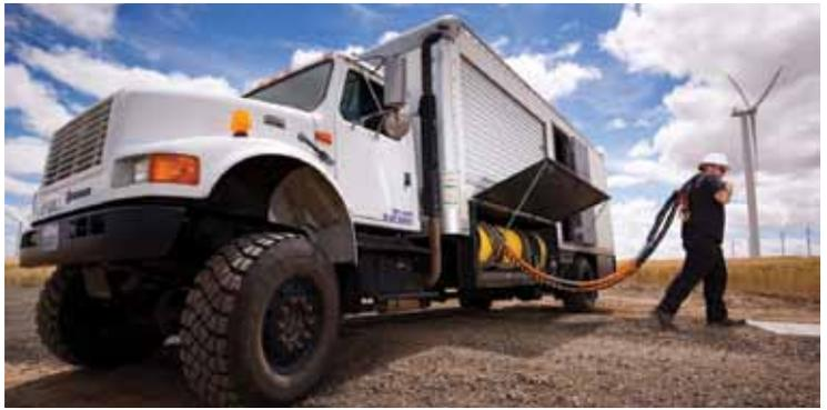
From the truck, this technology includes a wireless touch screen control system – sent via a truck-produced Wi-Fi signal – that eliminates any type of improper procedures taking place up tower. Depending on the filtration requirements of the customer (3, 5 or 10 microns), filters can be changed on the truck to accommodate the request. By using oil trays and pig mats, any residual spills can be contained.
