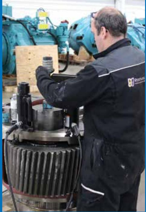
A Romax engineer disassembles planetary stage of a gearbox during failure root cause analysis.
