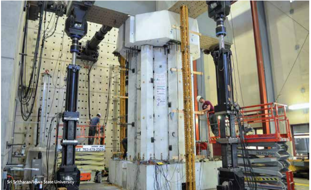
Iowa State doctoral student Robert Peggarr (right) helps prepare a Hexcrete cross section for load tests at the University of Minnesota's MAST Laboratory.
