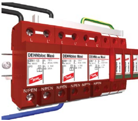
Fig. 2: Example of a combination of Class I and Class II SPD, using coordinated spark gaps and metal oxide varistors.
