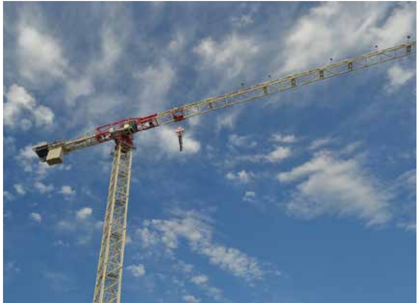
The Terex® CTT 472-20 flat top tower crane. (Courtesy: Terex)
