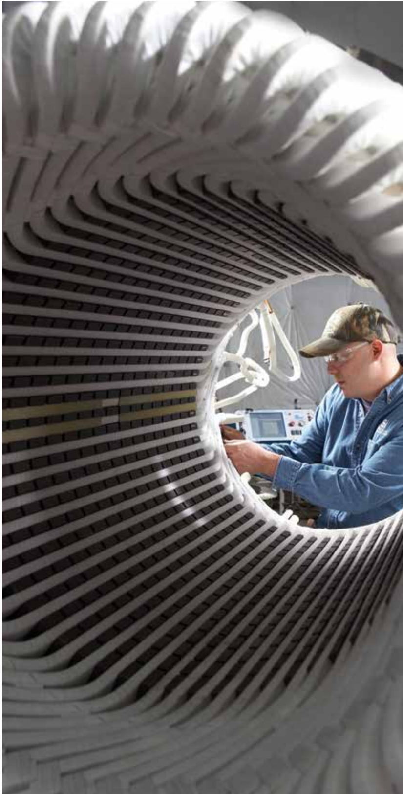
Stator during winding process.
