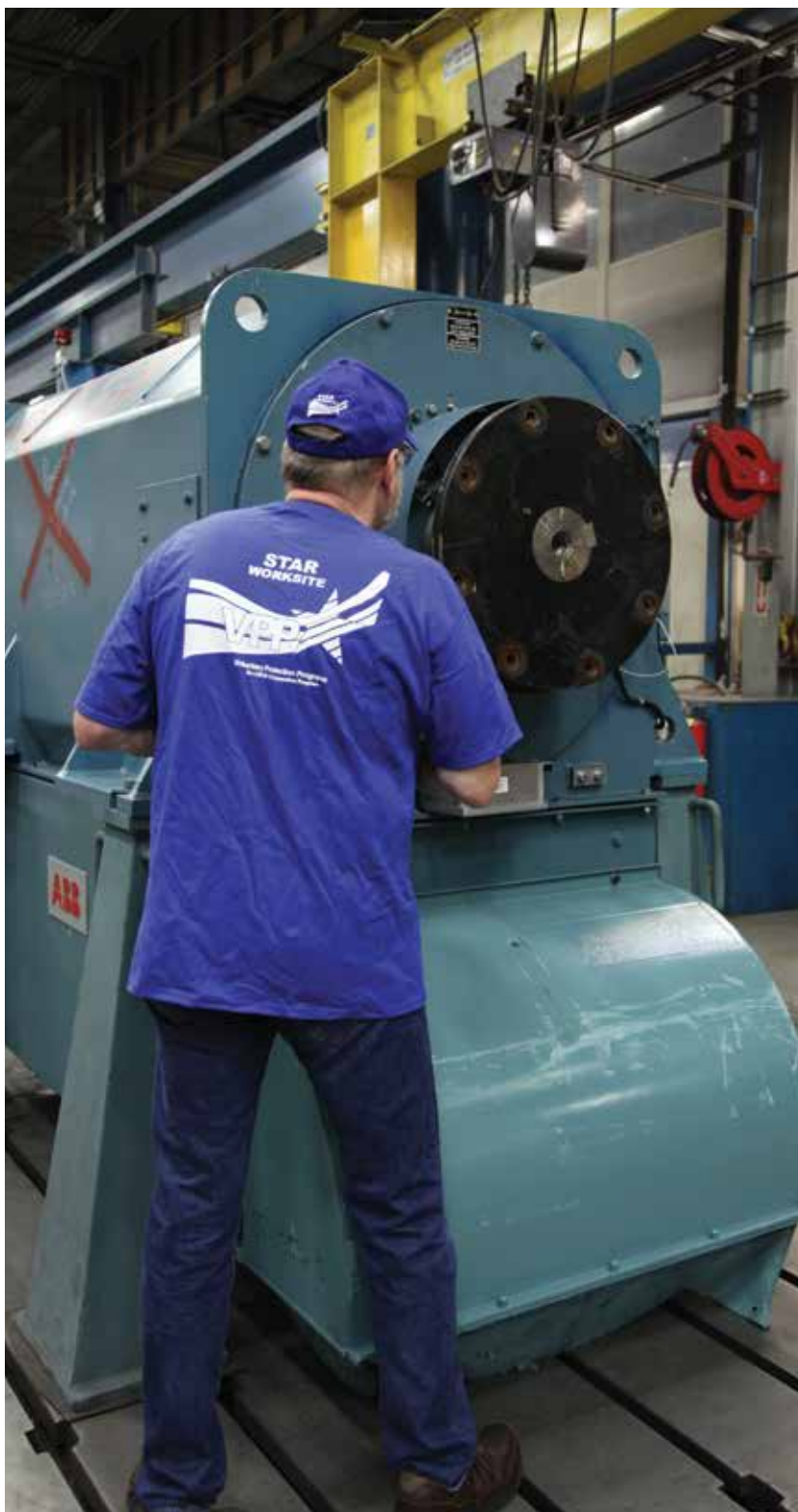
Remanufactured wind generator being set up for testing.
