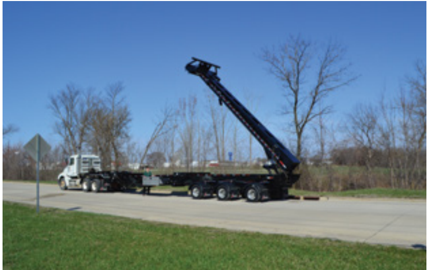
XL's 27-foot long Flip Extension can be added to the rear of XL's BladeMate trailer or any blade-hauling trailer. (Courtesy: XL Specialized Trailers)
