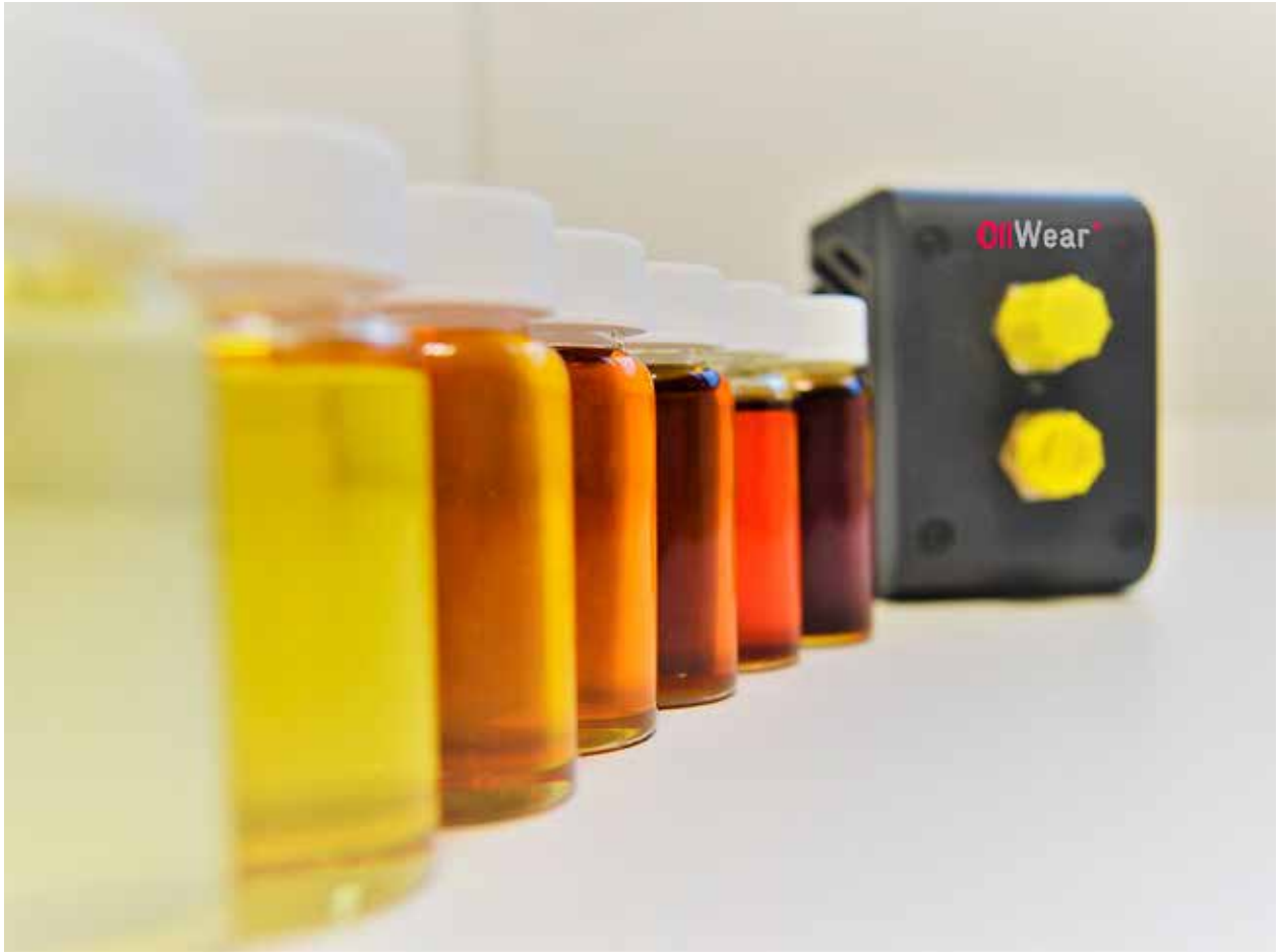
An optical sensor that monitors the state of lubricant oil. (Courtesy: Atten2)
