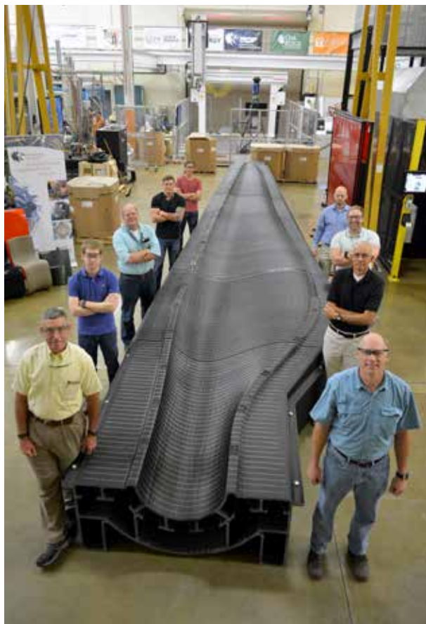
A group of researchers gather around a completed, 3D-printed blade mold. (Courtesy: Oak Ridge National Laboratory)
