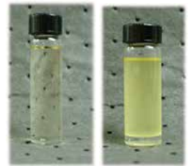
Hydrolytic stability shown: On the left is a PAG with 20,000 ppm water added, and it remains crystal clear. On the right is a PAO product. (Courtesy: American Chemical Technologies)
