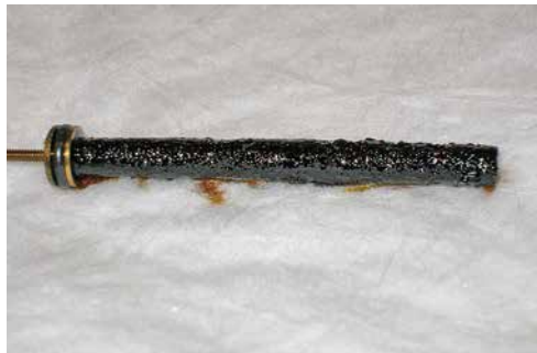
Typical varnish seen when running a PAO lubricant. (Courtesy: American Chemical Technologies)
