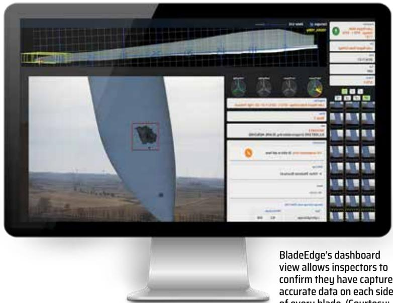
BladeEdge's dashboard view allows inspectors to confirm they have captured accurate data on each side of every blade. (Courtesy: BladeEdge)
