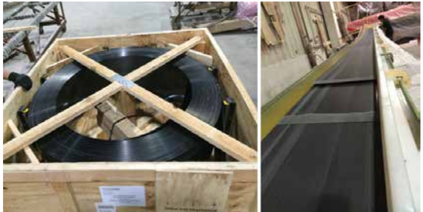
Pultrusion in the form of spooled strips and laminated as flat-plate creates a low-cost, high performance tapered spar. (Courtesy: TPI Composites)
