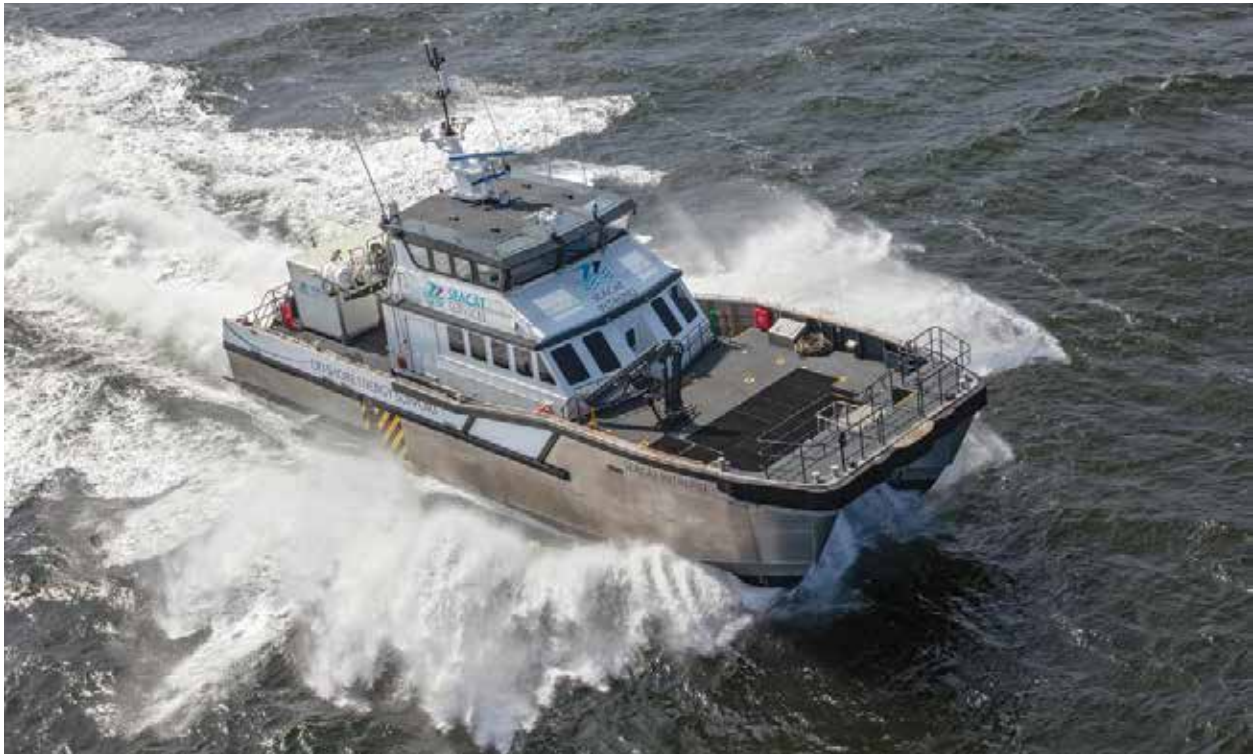
The Seacat Intrepid is a CTV used in offshore wind projects. (Courtesy: Seacat Services)
