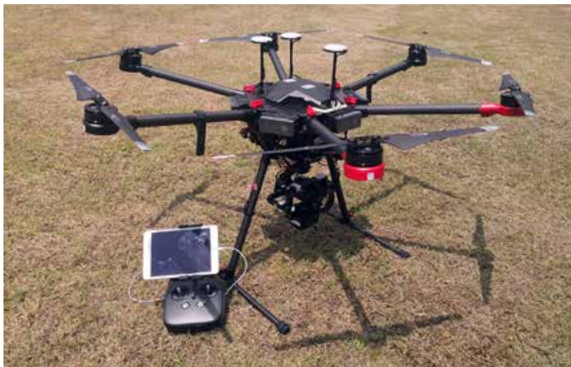
Clobotics gave “brains” and “eyes” to its drones, so the drones can see where the blades are as they fly and determine how to keep the blade within the center of the onboard camera and capture high-resolution photos in the air. (Courtesy: Clobotics)
