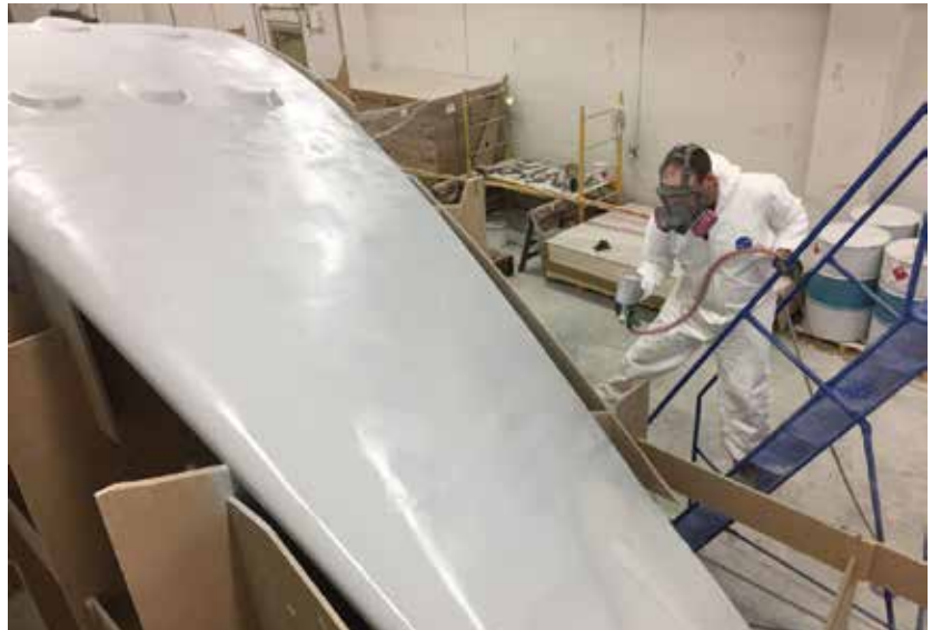
A PowerCone blade during fabrication. (Courtesy: Biome Renewables)
