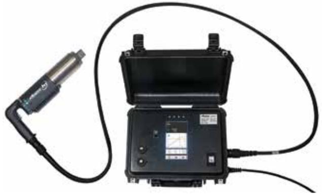
AcraDyne's IEC4W Field Controller/HT Nutrunner system is one example of a high-tech solution that ensures process repeatability and traceability in critical bolting. The tool's built-in transducer coupled with the powerful controller enables comprehensive tool programming and diagnostics, as well as real-time data analysis and troubleshooting. (Courtesy: AIMCO)
