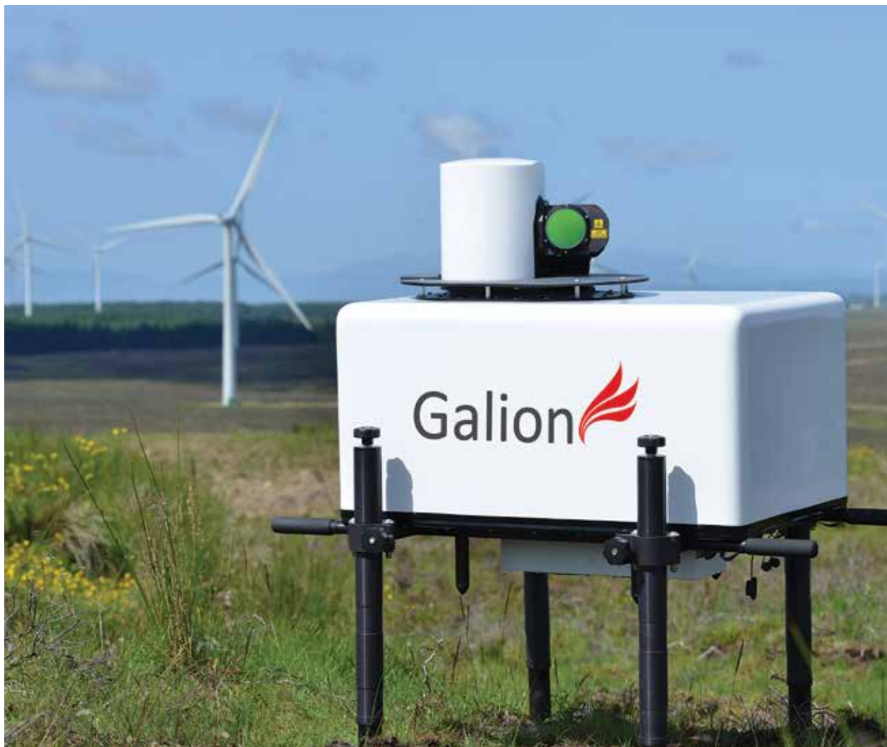
A Lidar device from Wood is helping a Swedish wind farm better understand the performance of both individual turbines and the overall estate. (Courtesy: Wood)
