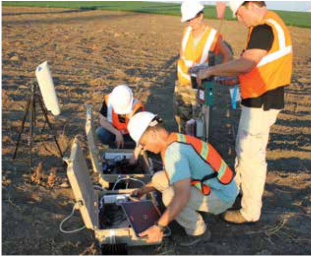
Thermal video cameras and acoustic detectors to record bat activity and behavior are installed at a wind turbine. (Courtesy: CanWEA)
