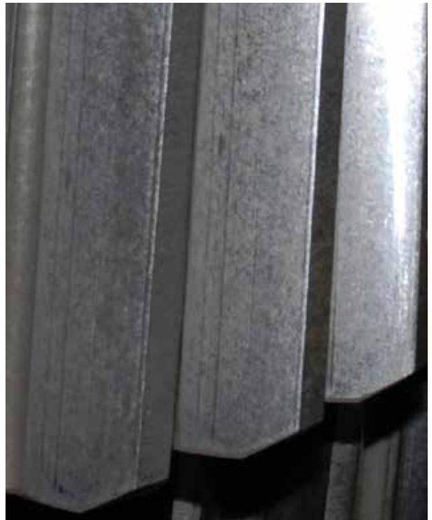
Figure 6: Closeup of the top planet after seven years showing no metal-to-metal contact pattern.
