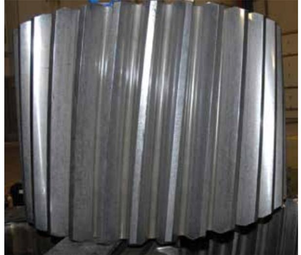
Figure 5: Three multi-megawatt class isotropic superfinished planets removed after seven years of operation.
