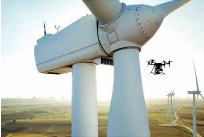
Based on the compact and flexible DJI M-210 drone, Sulzer Schmid's latest innovation delivers high performance and fully autonomous drone inspections. (Courtesy: Sulzer Schmid)
