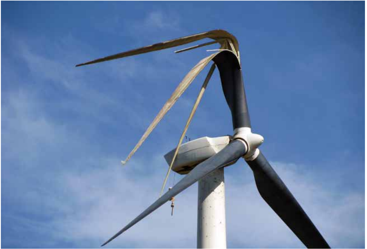
Although lightning can cause power surges that can be harmful to a turbine, most lightning damage occurs from dramatic heating of the composite blade materials. (Courtesy: Shutterstock)
