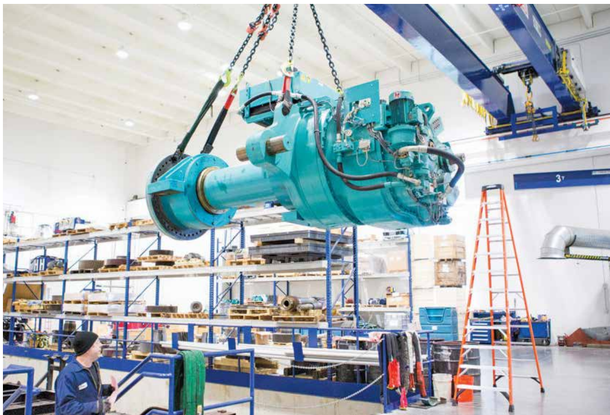
Gearbox Express is North America's largest independent remanufacturer of gearbox assemblies and main shafts for the wind-turbine industry. (Courtesy: Gearbox Express)
