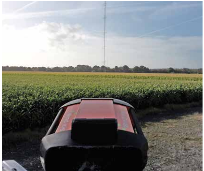
Nacelle Lidars have gained in importance in the last years — especially with regard to the verification of warranted power curves. (Courtesy: Deutsche WindGuard Consulting GmbH)
