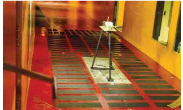
Figure 5: NASA's Glenn Icing Research Tunnel in Cleveland, Ohio. Modern ice sensors were originally developed for aircraft; tested here for compliance with SAE Aerospace Standard 5498 ¶5.2.1.1.1. (Courtesy: NAS)
