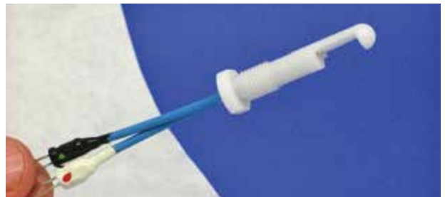
Figure 6: A fifth-generation ice detector protects wind-farm drones from hazardous ice during daytime and nighttime operations, helping to comply with FAA regulations. (Courtesy: NAS)
