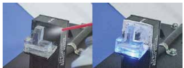
Figure 2: Modern ice sensors provide a local “ice alert” indicator for the convenience of technicians working aloft. (Courtesy: NAS)
