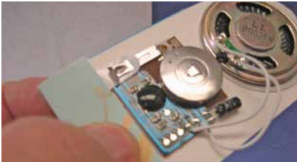
Figure 4: The 3/8-inch plastic dot in a musical greeting card contains more electronic functionality than a modern ice sensor. Custom chips like this are low cost and high quantity. This manufacturing technique promises deeply eroding sensor prices with increasing quantity. (Courtesy: NAS)
