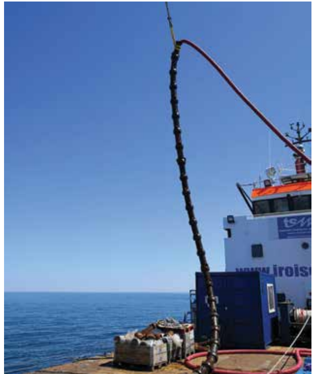
The use of cast iron for offshore ballasting shells ensures cable protection, stability, strength, and the best possible performance thanks to the mechanical properties of the material able to withstand the harshness of marine environments. (Courtesy: FMGC)
