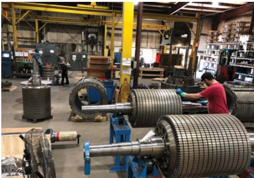
Several onshore wind generator sets get final production steps. (Courtesy: Sotek)
