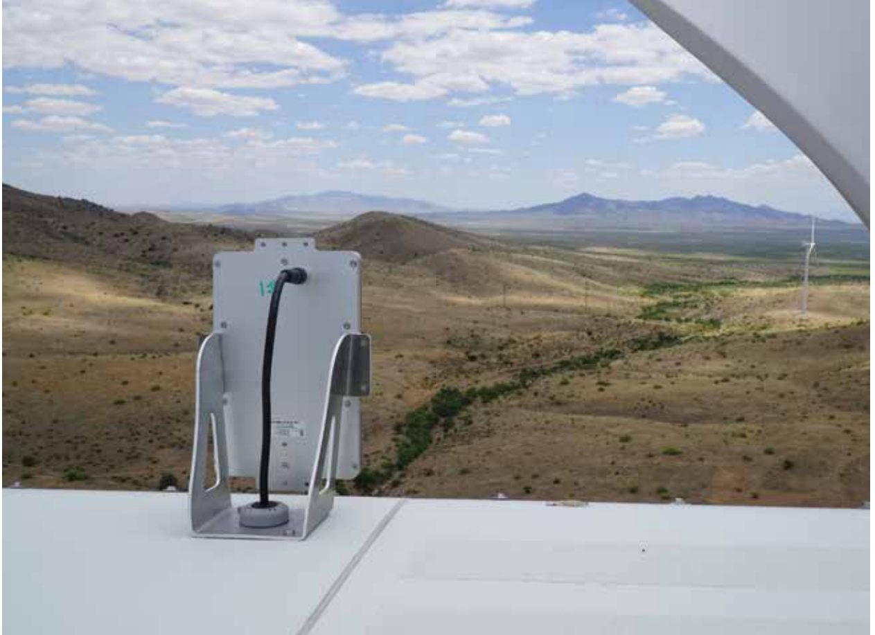
A Bat Deterrent Unit installed on a wind turbine at Red Horse 2. (Courtesy: NRG Systems)
