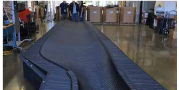
In 2017, TPI Composites concluded a joint research project with Oak Ridge National Labs (ORNL) and Sandia National Labs (SNL) that collaboration demonstrated the feasibility of large-scale AM in reducing production cost, time, and environmental impact of wind-turbine blade molds. (Courtesy: TPI Composites)
