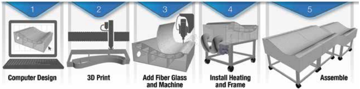
Process for 3D printing wind turbine blade molds. (Courtesy: TPI Composites)
