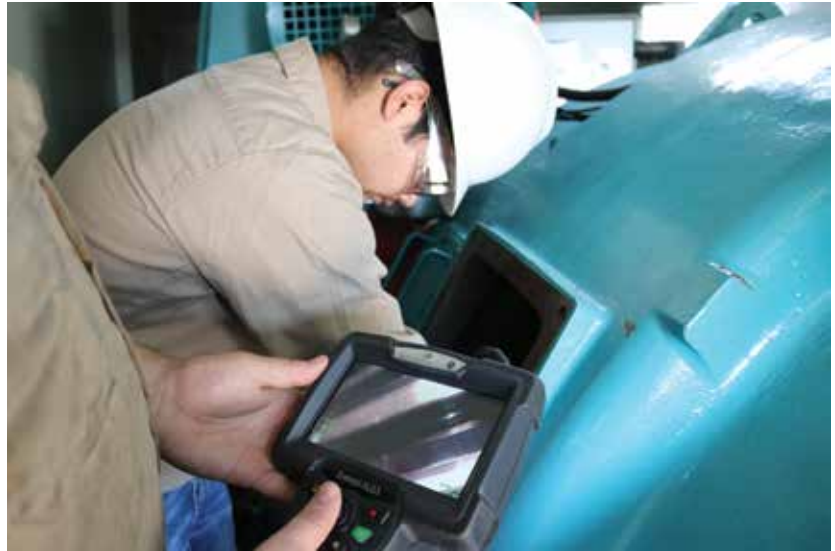
The borescopes allow students to use modern remote visual inspection techniques to learn how wind-generation equipment works. (Courtesy: NextEra)
