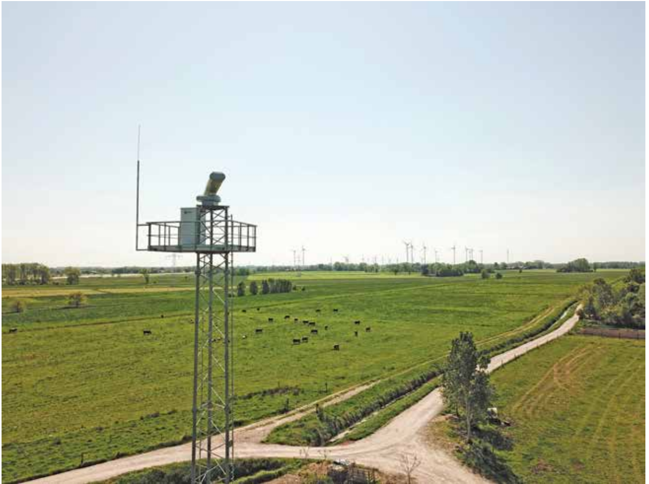
Terma's Obstruction Light Control (OLC) vastly reduces light pollution, and increases public acceptance of wind farms. (Courtesy: Terma)
