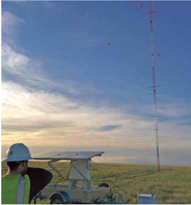
Lidar allows for accurate and more expansive measurements of the full wind profile in the development phase, helping determine the wind turbines to be selected and how much wind energy a future wind farm would produce. (Courtesy: Leosphere, a Vaisala company)
