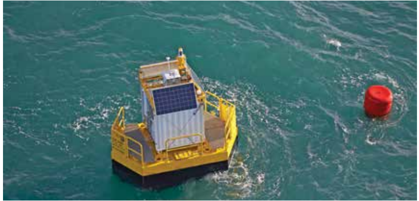
The buoy-ready Windcube’s new design will provide all of the innovation embodied in the Windcube but features a more robust casing in order to withstand difficult marine conditions in a moving platform at sea. (Courtesy: Vaisala/@Jacques Vapillon-AKROCEAN GEPS Techno)
