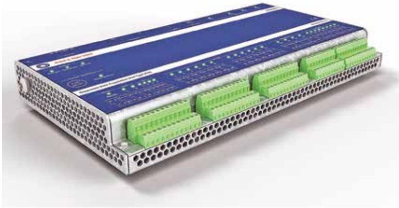
A BKV diagnostic data acquisition unit. (Courtesy: BKV)
