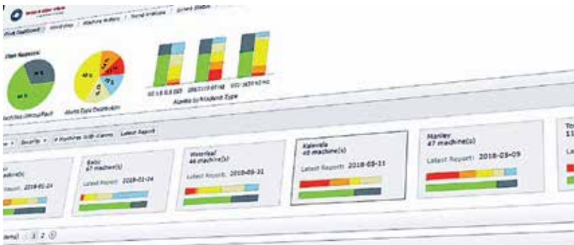
VibroSuite enables advanced diagnostics to be done on the time waveform data for the individual wind turbine and drive-train components, as well as used for turbine performance comparison through fleet monitoring. (Courtesy: BKV)
