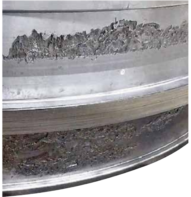
Figure 2: Spalling on the gear-box side of a wind turbine main shaft bearing: the result of uneven load conditions.
